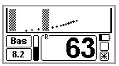
After pressing the will button the « Sensitivity » message will appear on the display, a number describing the Sensitivity level and a linear scale showing the adjustment range. The adjustment is done using the sensitivity buttons. Pushing the will button a second time will show the Discrimination level. Adjusting the Discrimination is done in the same way as adjusting the Sensitivity.
