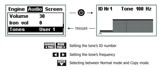
After selecting a suitable sound profile from the User group it can be edited by pressing the button. The buttons are used to choose the ID number for which a specific tone is applied and the buttons are used to change the frequency of the sound. The ID number currently edited is shown by a digit and a cursor (a filled triangle for the Copy mode and an empty one for the Normal mode) which are shown at the bottom of the display.
